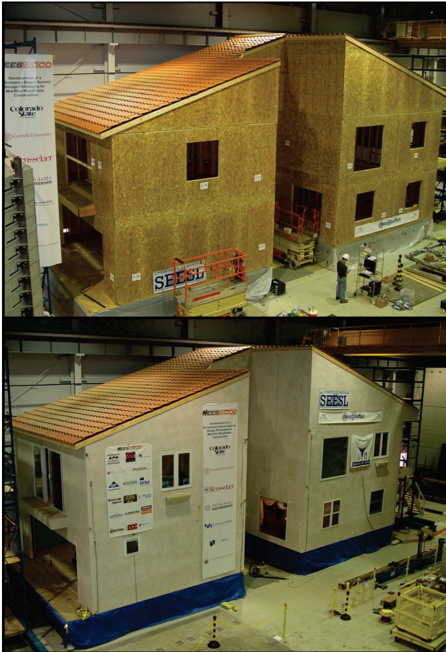
Figure 2-20 CUREE-Caltech Woodframe Project test building on the SEESL shake tables: Test Phase 1 (SFRS only) configuration (top); and Test Phase 5 (SFRS with interior gypsum board and exterior stucco finishes) configuration (bottom) (Filiatrault et al., 2010).
