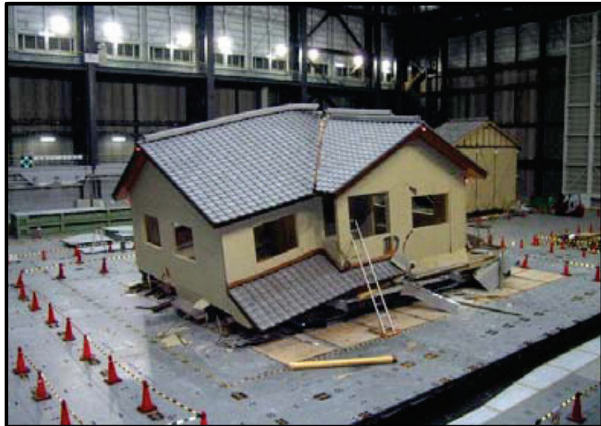
Figure 2-18 Collapsed test building after the third JR Takatori shake (Isoda et al., 2008).
